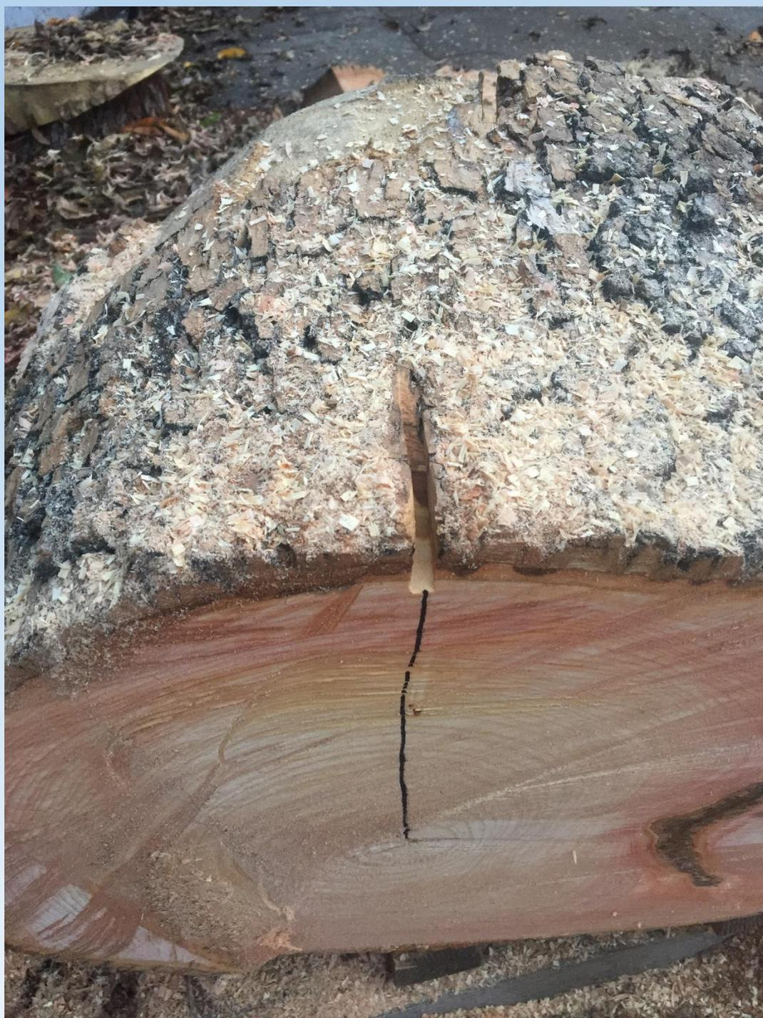
*Drawing a vertical line on the opposite end and cutting a nick there will allow you to align the saw with the nicks and make a vertical cut down both lines.*
