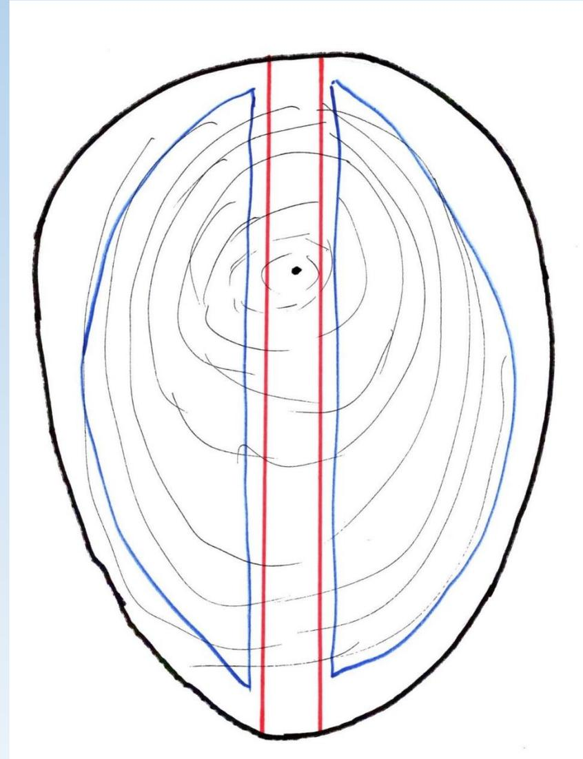
When cutting the pith out of the log, it is possible to leave enough material in the middle to allow for two platter blanks. You will also want to make a cut to flatten the base of the bowl blanks.
