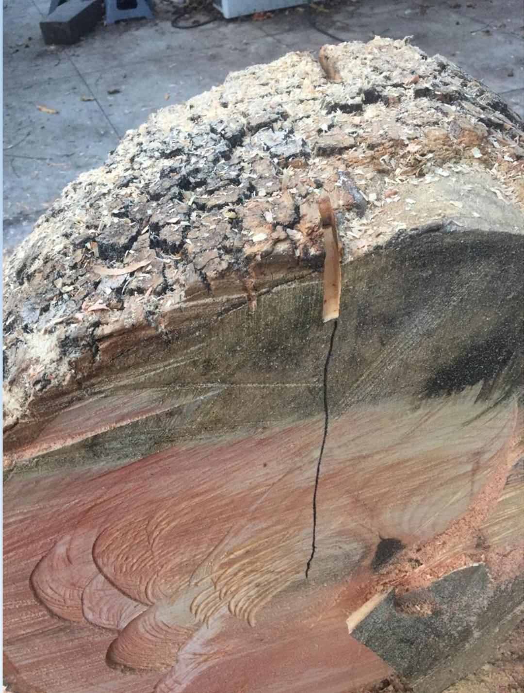
If you stop short of completing your cuts, the log will remain stable. Once both cuts are almost finished you can go back and finish them. This reduces the amount of work on an unstable blank.
