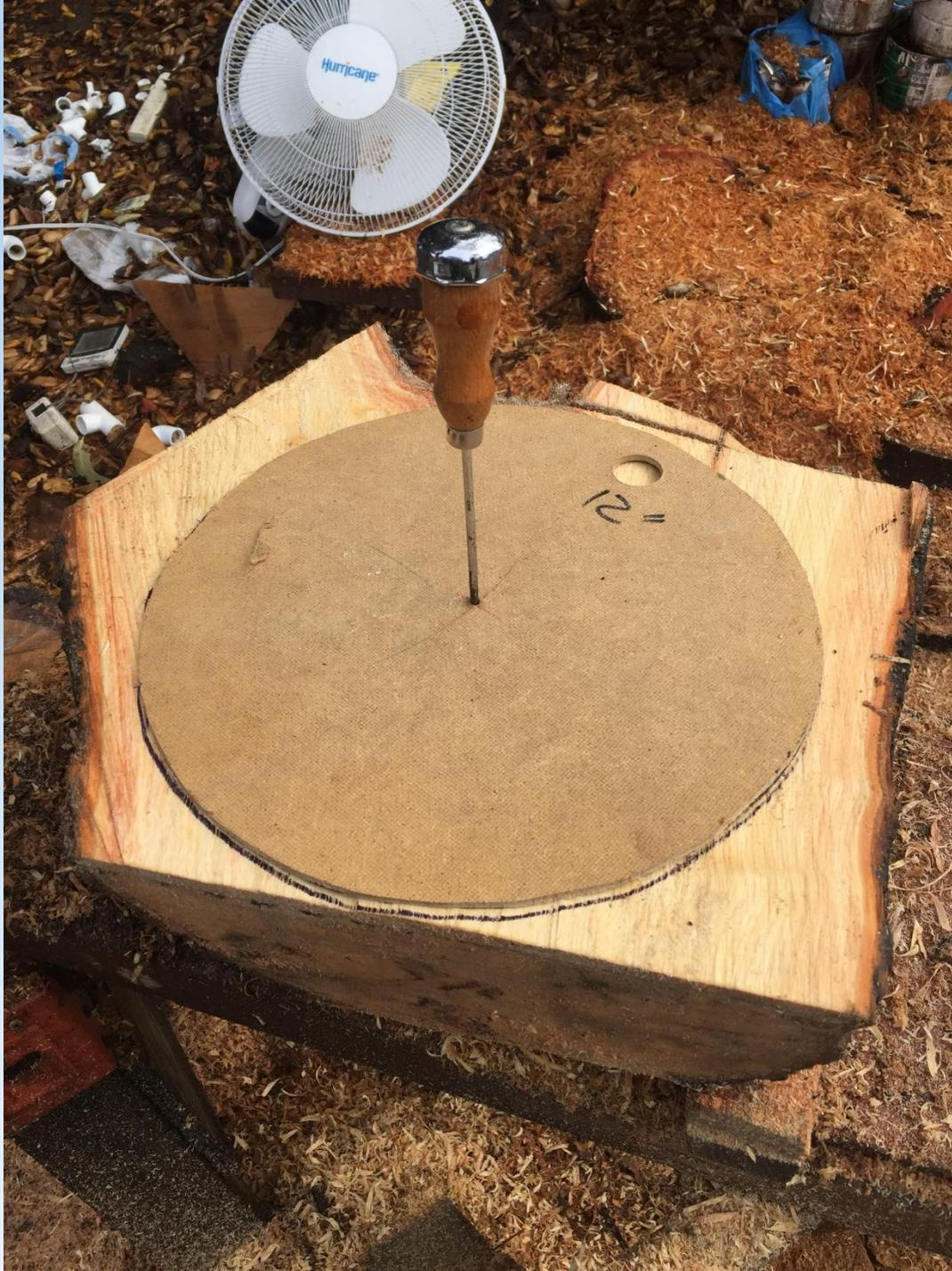
*Use the chainsaw to make a number of cuts close to the circle to produce a near-round blank.*
