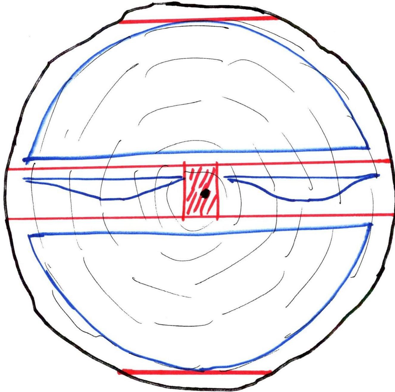
Once you have the blanks cut round, it helps to cut off the two “ears” on each end. This will save a lot of grief when turning the bottom of the bowl blank. The image on the right has the “ears’ cut off.
