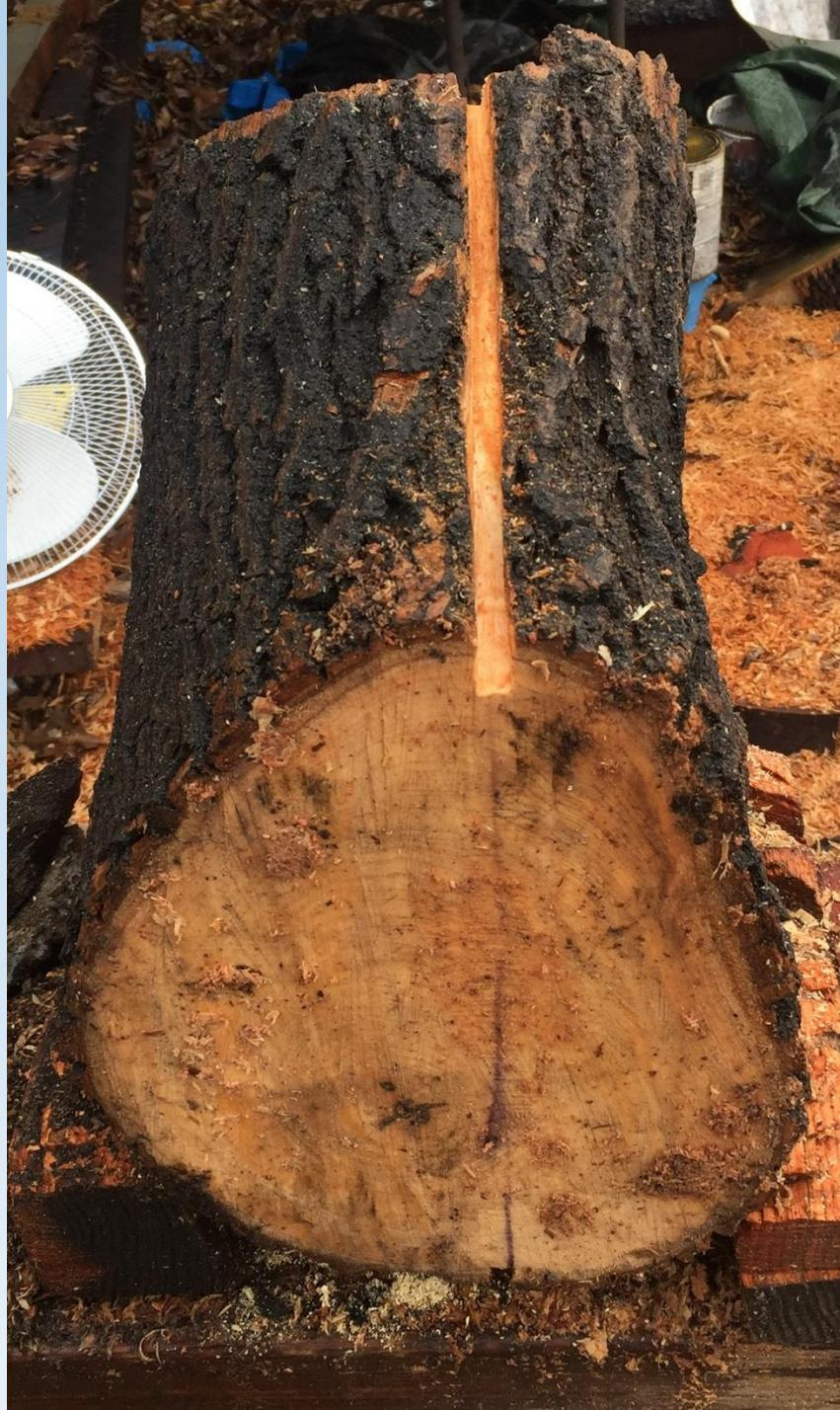
Bowls and platters made from crotch blanks need to be turned with rim on the bark side of the blank. Otherwise you will be turning out all the figure.
