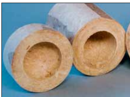
Allow the roughed-out pieces to rest a few days, which will reduce the amount of wood movement due to hollowing.
