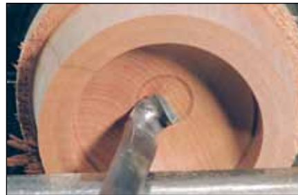
Inside the lid, the hook tool performs two actions: working with the grain and cutting the wood.
