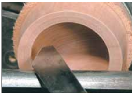
Cut the mortise shoulder with an offset diamond scraper and a shear-scraping action. Be sure not to sand this area.
