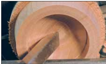
If you don't have a hook or ring tool, use a 1/2" roundnose scraper in a shear-scraping action to finish the end-grain. Tilt it to the left to about 45 degrees.
