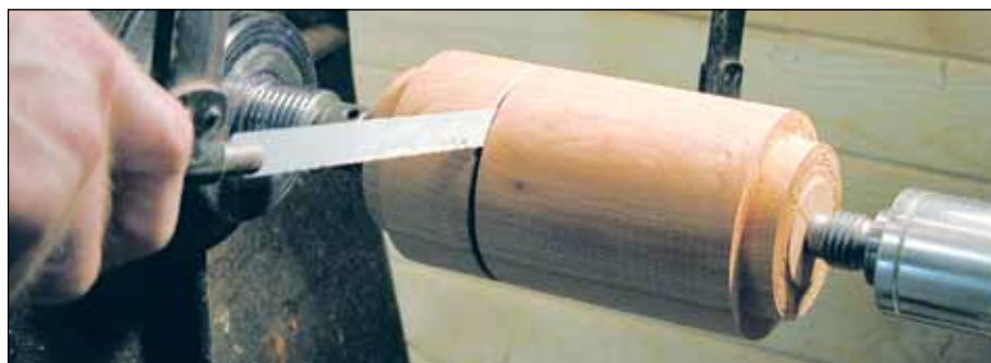
Use a hacksaw (teeth pointing away) in a heavy frame to minimize wood loss in separating the lid from the base. This will improve grain flow between the two parts.
