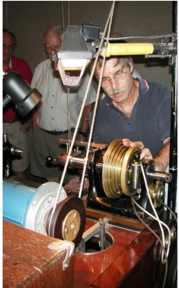
Jim working at the Holtzapffel. The belt in the foreground goes to an overhead transfer above and then, via another belt, to the crossfeed toolrest.
