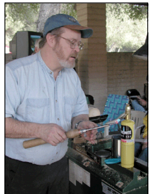
Alan Lacer shows how to anneal a cutting tool
