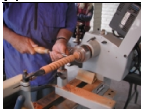
Bill Kelly, chiseling out the space between the bines.
