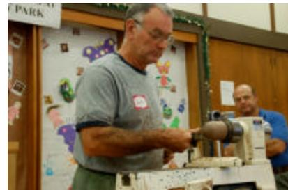
Jim O'Connor, past president, gave us a different way to make a round ball. He was well prepared with pre-turned examples of different steps in his process which made the demo go along at a very fast clip. In his hand-out he shows using a vblock to hold the turned cylinder but in the demo he just used his chuck with the short
