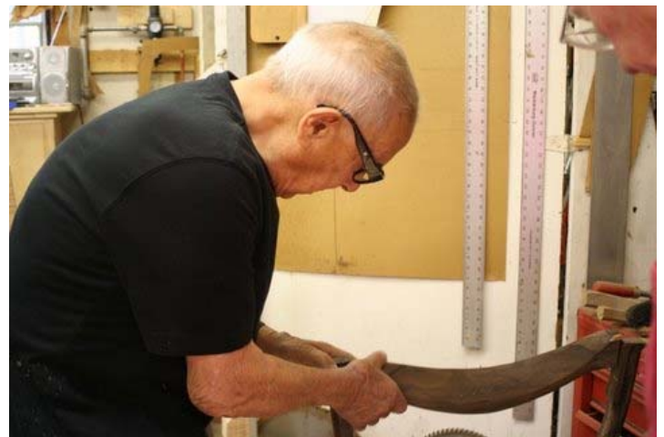
Sam demonstrating the fit of a chair arm that he just cut for us on the band saw.
