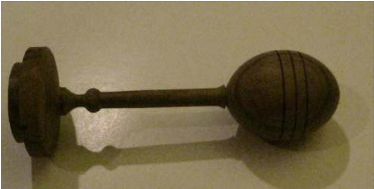
Finish cutting the bead end off of the waste stock. Clean up the end of the handle and sand by hand to remove the last little bit.
