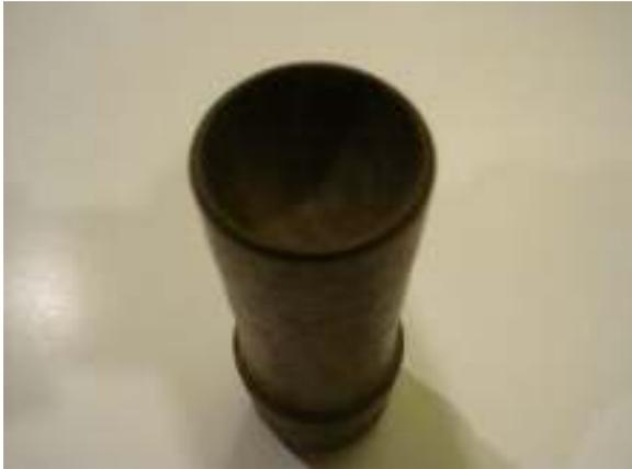
Remove the piece from the main body and set aside. Clean up the face of the main body and cut a mortise to accept the  $1/16 \times 1/16$  tenon on the top piece. Use the live center in the tailstock to hold the top piece in place and turn the outside shape of the top, removing the top periodically to check your wall thickness. Leave a small nub on the end where the center is. When finished set the top aside.
