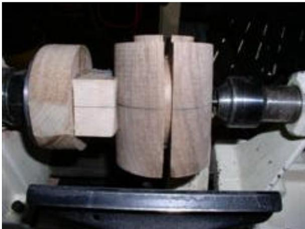
You can use a v-block as shown in the diagram for the head stock to hold the cylinder 90° from between centers as shown or it is much easier to open the jaws on your chuck to simulate a v-block. The better centered the cylinder is the easier it is to get a good sphere, but it will work even if you are slightly off. The tail stock
