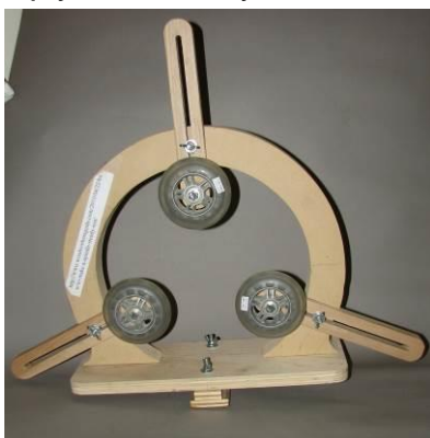
John Janssen brought in a vase turned out of mystery wood and finished with Minwax Polycrylic. He also brought in a steady rest that he made in order to help him turn the vase. It was made from MDF, Birch ply and Cherry.
